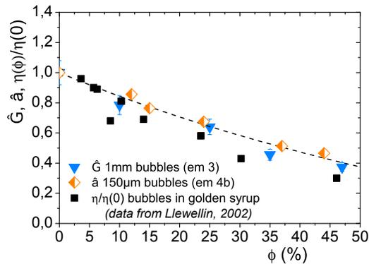
Figure 5: Dimensionless viscosity (bubbles in a Newtonian liquid, data replotted from Llewellyn et al. (2002)), dimensionless reduced dissipation  $\hat{G}''$  and dimensionless elastic modulus (both, bubbles in a yield stress fluid) as a function of  $\phi$ . The dashed line is, as before, the result of equation 2 in the limit case of  $Ca \rightarrow \infty$ .
