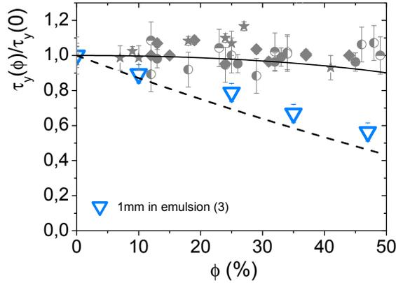
Figure 7: Dimensionless yield stress as a function of the gas volume fraction, for  $R = 1$ mm bubbles in emulsion 2. The grey symbols are all the other systems, re-plotted here for comparison. The dotted line is the theoretical limit given by equation 9.
