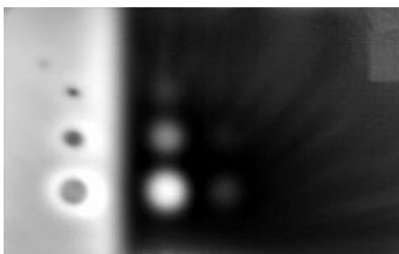
Figure 9. Lock-in IRT in specimen A
