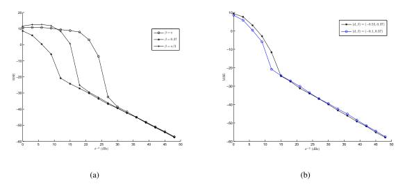
Fig. 2. (a) The MSE curves with different values of  $\beta$  with fixed d=-0.1 in the case of white Gaussian noise. (b) MSE curves comparing the performance between the optimization (15) and the proposed algorithm in the case of white Gaussian noise.
