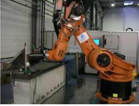
Fig. 1. Robot KUKA KR500 MT-2 (by courtesy of Institut de Soudure)
