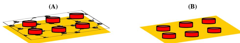
**Fig. 1** Schematic illustration of the different interfaces investigated: (A) graphene coated Au thin film decorated with Au NPs array; (B) Au NPs array directly deposited onto thin Au film without the graphene spacer layer.
