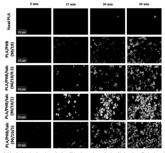
Figure 7. Selected polarization photomicrographs of neat PLA, and composites as a function of isothermal crystallization time at 130°C.
