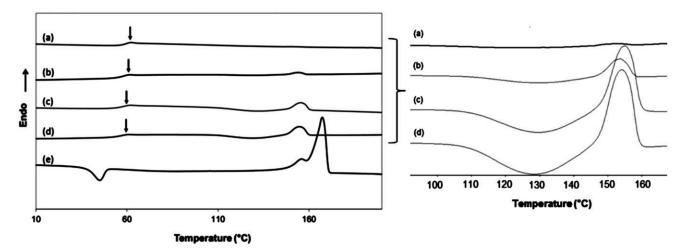
Figure 1. DSC thermograms obtained from the second heating runs with a heating rate of 10°C min<sup>-1</sup> of neat PLA (a), PLA/PHB (95/5) (b), PLA/PHB (90/10) (c), PLA/PHB (80/20) (d), neat PHB (e), with a zoom around the cold-crystallization peak of PLA.
