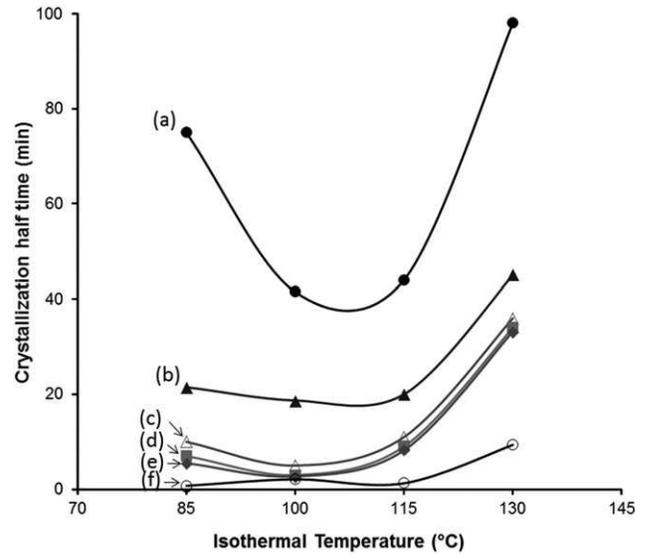
**Figure 6.** Isothermal-crystallization half time ( $t_{0.5}$ ) for neat PLA (a), PLA/PHB (90/10) (b), PLA/PHB/talc (90/10/0.5) (c), PLA/PHB/talc (90/10/1) (d), PLA/PHB/talc (90/10/5) (e) and neat PHB (f) as a function of isothermal temperature.
