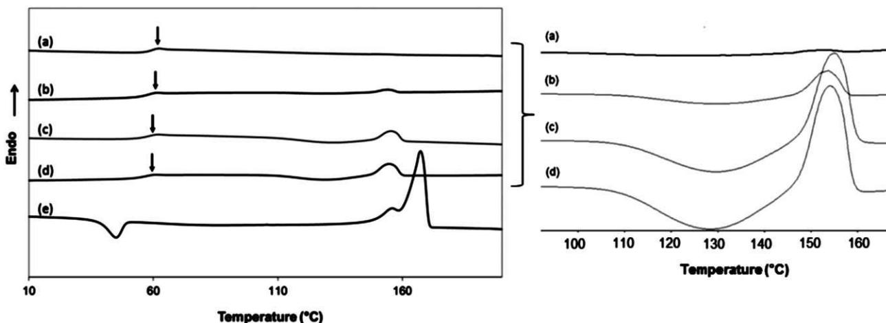
**Figure 1.** DSC thermograms obtained from the second heating runs with a heating rate of  $10^{\circ}\text{C min}^{-1}$  of neat PLA (a), PLA/PHB (95/5) (b), PLA/PHB (90/10) (c), PLA/PHB (80/20) (d), neat PHB (e), with a zoom around the cold-crystallization peak of PLA.
