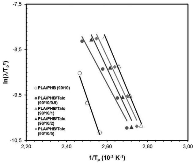
**Figure 5.** Plots of  $\ln(\lambda/T_p^2)$  versus  $1/T_p$  during nonisothermal cold crystallization process for PLA/PHB (90/10), PLA/PHB/talc (90/10/0.5), PLA/PHB/talc (90/10/1), PLA/PHB/talc (90/10/2), PLA/PHB/talc (90/10/5).
