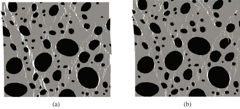
Fig. 15: Deformed specimens for confinement pressures of (a) 3 Mpa and (b) 6 MPa. Displacement has been magnified by a factor of 5 .
