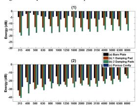
Figure 9. Numerically obtained subsystem energy levels in 1/3 octave bands for case (a), (b) and (c). (1) Plate subsystem energy. (2) Cavity subsystem energy
