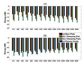
Figure 10. Experimentally obtained subsystem energy levels in 1/3 octave bands for case (a), (b) and (c). (1) Plate subsystem energy. (2) Cavity subsystem energy
