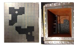
Figure 2. Two damping pads attached to a steel plate (left). A porous material inside a cavity (right)
