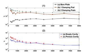
Figure 7. Experimentally estimated subsystem damping loss factors averaged in 1/3 octave band for case (a), (b) and (c). (1) Plate subsystem damping. (2) Cavity subsystem damping.
