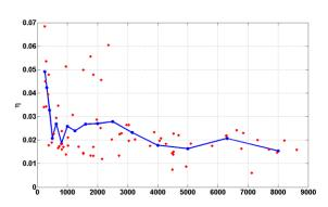
Figure 6. Damping loss factors of the plate treated with a single damping pad (case (b)). The red dot are damping levels of individual modes, and the blue line is an average value in 1/3 octave band.
