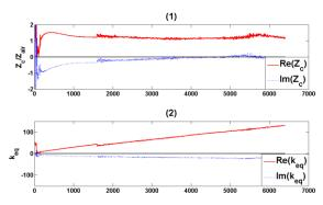
Figure 4. Complex equivalent parameters of the porous material. (1) Normalized characteristic impedance. (2) Fluid wavenumber
