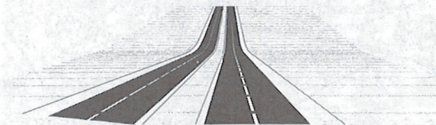
Transition of a 2% downgrade to a 3% upgrade effected by the minimum curve for 70 mph. The curve is 700 feet long, vertical radius about 14,000 feet.
