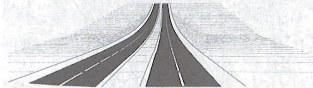
Transition of a 2% downgrade to a 3% upgrade effected by a liberal curve 3,000 feet long, vertical radius about 60,000 feet.
