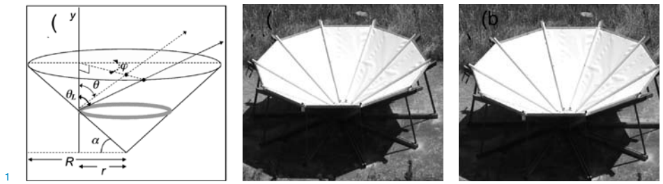
Figure 1 Integration scheme for the funnel shape ( 0 < \theta < \theta_L , 0 < \phi < 360^\circ and 0 < r < R ). (b) Photo of the funnel-shaped condenser ( 7.3 \text{ m}^2 surface area with 60^\circ cone angle, 30^\circ from horizontal). The internal surface of the experimental condenser is coated with OPUR ( www.opur.fr ) low density polyethylene film insulated from below with 3 cm styrofoam.
