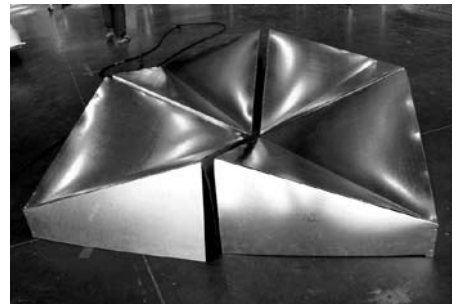
Figure 5 Inverted pyramid with an angle 30^\circ from horizontal and four condensation side. The section at the top is 1\text{ m} \times 1\text{ m} .
