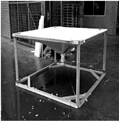
Figure 5 Inverted pyramid with an angle 30^\circ from horizontal and four condensation side. The section at the top is 1\text{ m} \times 1\text{ m} .
