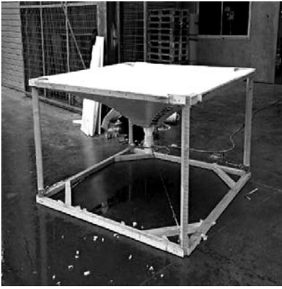
Figure 5 Inverted pyramid with an angle 30^\circ from horizontal and four condensation side. The section at the top is 1 m x 1 m.
