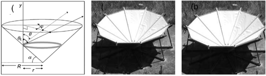
Figure 1 Integration scheme for the funnel shape ( 0 < \theta < \theta_L , 0 < \phi < 360^\circ and 0 < r < R ). (b) Photo of the funnel-shaped condenser ( 7.3 \text{ m}^2 surface area with 60^\circ cone angle, 30^\circ from horizontal). The internal surface of the experimental condenser is coated with OPUR ( www.opur.fr ) low density polyethylene film insulated from below with 3 cm styrofoam.
