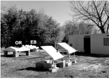
Figure 7 "Egg Box" (EB) and "Origami" (OR) type condensers with the planar reference condenser (R). (T is an additional planar condenser).
