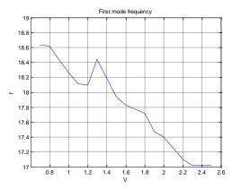
Figure 5. Identified first modal frequency depending on fluid velocity (m/s)
