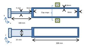
Figure 2. Gap supported tube
