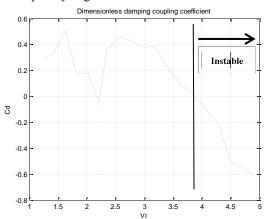
Figure 7. Identified dimensionless fluid-elastic damping coupling coefficient depending on dimensionless reduced fluid velocity
