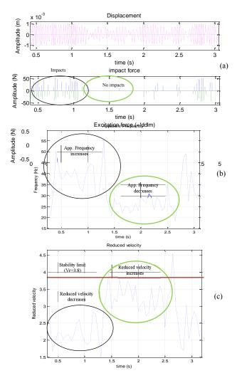
Figure 9. (a) Tube response & estimated impact force (b) Apparent frequency (c) Reduced velocity
