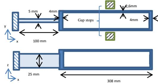
Figure 2. Gap supported tube
