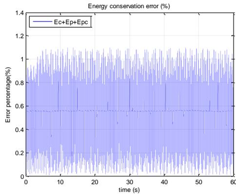
Figure 11. Newmark with Newton Raphson method conservation energy error
