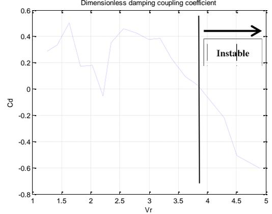
**Figure 7. Identified dimensionless fluid-elastic damping coupling coefficient depending on dimensionless reduced fluid velocity**
