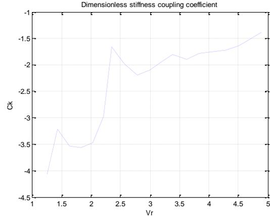
**Figure 8. Identified dimensionless fluid-elastic stiffness coupling coefficient depending on dimensionless reduced fluid velocity**
