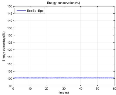
Figure 10. Newmark with Newton Raphson method conservation energy
