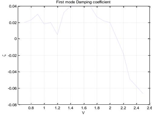
**Figure 6. Identified first modal damping coefficient depending on fluid velocity (m/s)**
