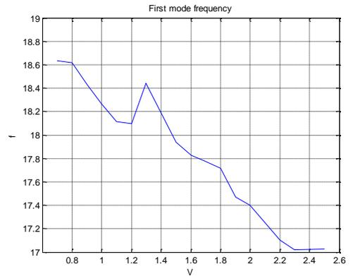
Figure 5. Identified first modal frequency depending on fluid velocity (m/s)
