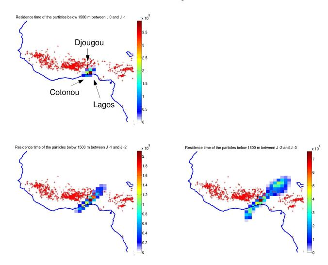
**Fig. 8.** Retroplumes calculated by the FLEXPART model for the first 24 h (top panel), between 24 and 48 h (bottom left), and between 48 and 60 h (bottom right) initialised over Cotonou in the ozone enhanced layers (between 800 and 1600 m) measured on the 20 December 2005. Black dots mark the position of Cotonou, Djougou and Lagos. Red crosses mark the position of active fires as detected by MODIS on the 16, 17, 18 and 19 December 2005.
