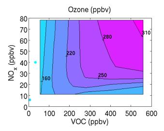
Fig. 10. Isopleths of the ozone concentrations as a function of  $\mathrm{NO}_{\mathrm{X}}$  and VOCs concentrations. This is interpolated from the calculation of 49 sensitivity tests using the box model as done for the so called additional petrochemical accident run.
