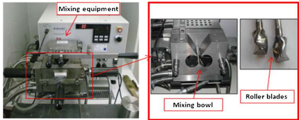
Fig. 3 The mixing equipment and its internal structure for mixing test
