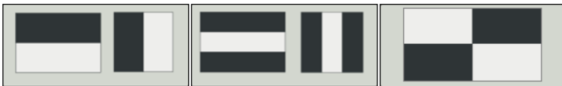
Figure 2-1 : Example of masks used in Viola and Jones algorithm
