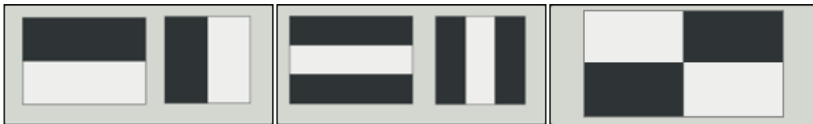
Figure 2-1 : Example of masks used in Viola and Jones algorithm
