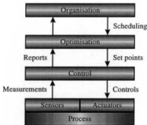
Fig. 2. CIP breaking up of industrial plant.
