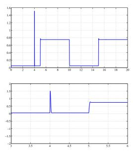
Fig. 12. Simulation of the non linear closed loop system with incremental controller, ouput y(t) (top), zoom on the output y(t) (bottom)
