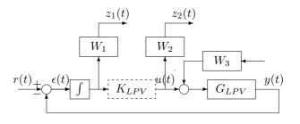
Fig. 2. Augmented plant corresponding to a modified four-block  $\mathcal{L}_2$  gain criterion
