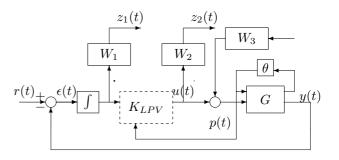
Fig. 9. Augmented plant corresponding to a modified four-block  $\mathcal{L}_2$  gain criterion
