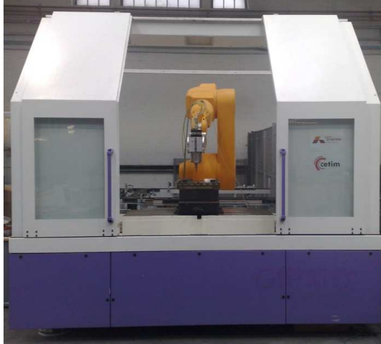
Fig. 1. Machining robot with high-speed spindle.
