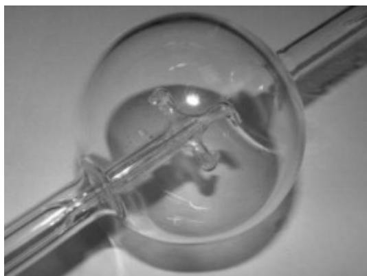
Figure 2: Jet-stirred reactor (JSR) used to study the gas-phase conversion of anisole.
