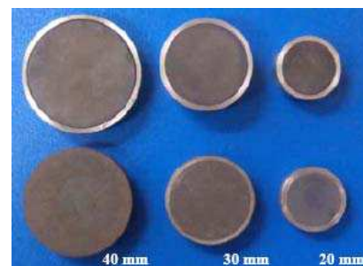
Fig. 1. Overview of the prepared bulk MgB 2 samples for the trapped field
