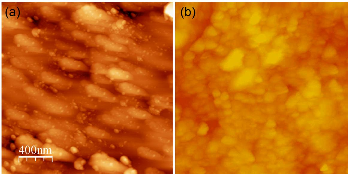
**Fig.2** AFM topography images (tapping mode) of the MgB<sub>2</sub> sample prepared at 775 °C (a) and of the sample prepared at 850 °C (b).
