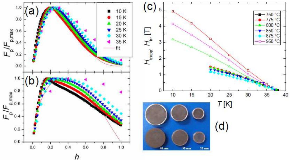
**Fig.1** (a,b) Pinning force scaling for the sample prepared at 950 °C (a) and 775 °C (b). The shown fits are fits to all data. The strong non-scaling of (b) is clearly visible. (c) gives the irreversibility lines (open symbols) and the measured trapped fields (full symbols). Finally, (d) illustrates the bulk samples prepared.
