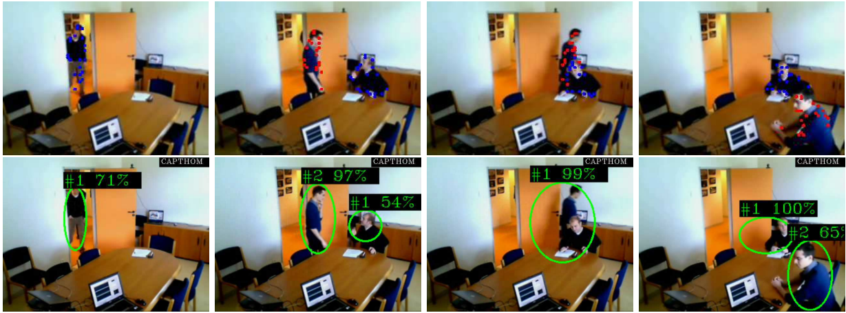
Figure 3: Illustration of tracking results with transient partial occlusion. The first line corresponds to input images with interest points associated with each object (one color per object), the second line presents the tracking result with the label obtained for each tracked object.
