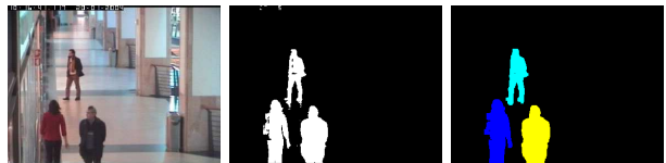
Figure 2: From the left to the right: original image, result obtained after background subtraction and finally after connected components gathering.
