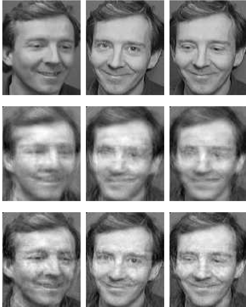
Figure 7: First line: 3 appearances of a face. Second line: PCA representation. Third line: NLPCA representation.
