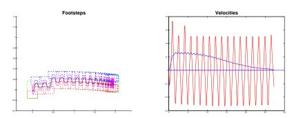
Fig. 3. Perturbation on a PBVS experiment for the humanoid robot reactive walking. A brutal pushing of the robot occurs close to (0.5, 0.2).
