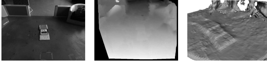
Fig. 4: From a pair of images of the scene in front of the robot (left) a dense disparity map is estimated (middle) and from this disparity map a dense surface integrating the previous frames into the volumetric grid is estimated (right). These images were taken from the HRP-2 stereo vision system with the cameras tilted towards the ground to allow ground reconstruction tasks. 4 It is assumed that a mechanism is implemented to make the robot search for traversable areas. 20
