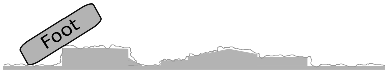
Fig. 5: Example of a situation handled by our pattern generator with the inverse dynamics stack of tasks. The gray part represents the real environment, and the green line the stereoscopic reconstruction. The foot is in its final position after the adaptation by the proposed method.
