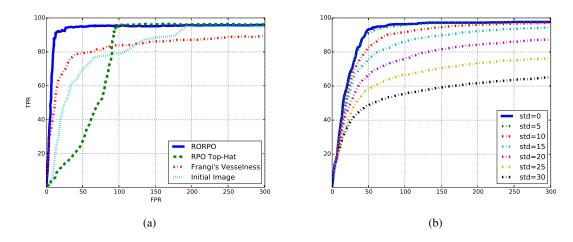
Figure 6: ROC curves on synthetic data. (a) Comparison of the three filters, plus the native image. (b) Noise robustness of the RORPO filter.
