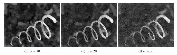
Figure 7: (a–c) Synthetic image for various amounts of Gaussian noise: maximum intensity projection. (d–f) Corresponding filtered images.
