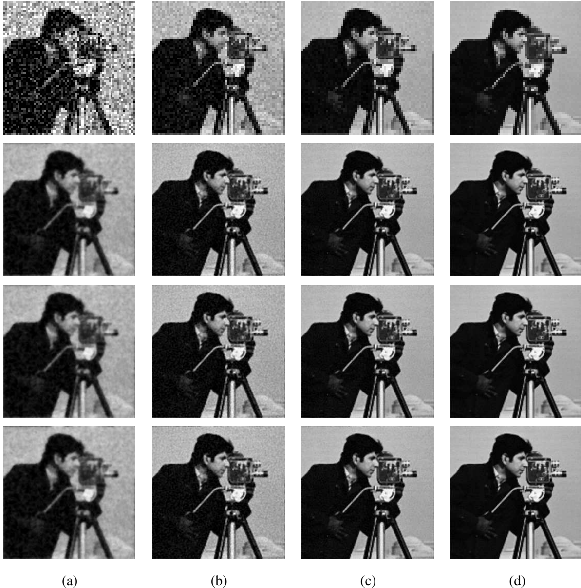
Fig. 1: One of the LR images (top row), HR images obtained by VBA-SR (the second row), EGrad-SR (the third row), Proposed approach (bottom row) for the Cameraman in the cases where SNR = (a) 5 dB; (b) 15 dB; (c) 25 dB (d) 35 dB. All images are presented in the same range of grayscale.
