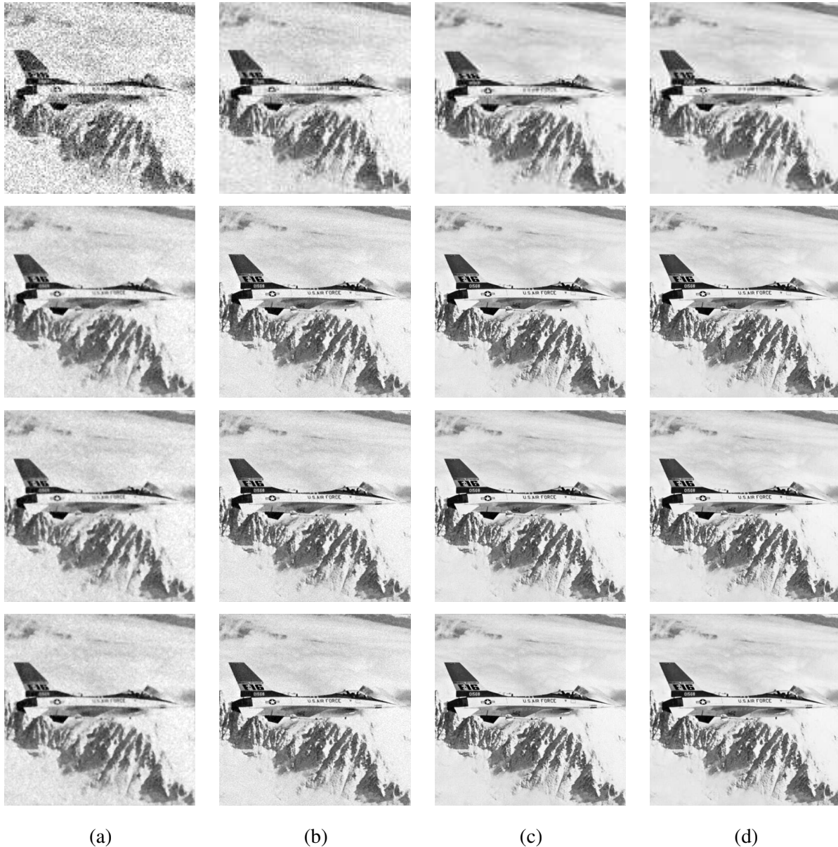
Fig. 2: One of the LR images (top row), HR images obtained by VBA-SR (the second row), EGrad-SR (the third row), Proposed approach (bottom row) for the Jetplane in the cases when SNR = (a) 5 dB; (b) 15 dB; (c) 25 dB (d) 35 dB. All images are presented in the same range of grayscale.
