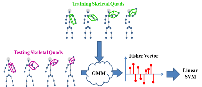
Fig. 1. A Gaussian Mixture Model (GMM), learnt on training data, is supposed to generate skeletal quads. Based on the GMM parameters, the skeletal quads of any action example are encoded into a Fisher vector, thus building the action descriptor which is led to a multi-class linear SVM.
