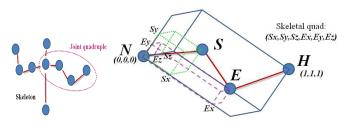
Fig. 2. An example of coding the marked joint quadruple {Neck, Shoulder, Elbow, Hand}. The Neck and Hand joints are identified with the points (0,0,0) and (1,1,1) in the new local coordinate system. The local 3D coordinates of the Shoulder and Elbow joints describe the structure of the quadruple and the quad descriptor is  $\mathbf{q} = [S_x, S_y, S_z, E_x, E_y, E_z]^T$ .
