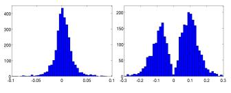
Fig. 3. The distribution of entries (left) before and (right) after the power normalisation ( $\alpha=0.5)$  of Fisher vector.
