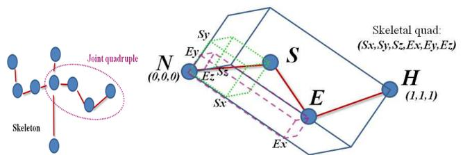
Fig. 2. An example of coding the marked joint quadruple {Neck, Shoulder, Elbow, Hand}. The Neck and Hand joints are identified with the points  $(0, 0, 0)$  and  $(1, 1, 1)$  in the new local coordinate system. The local 3D coordinates of the Shoulder and Elbow joints describe the structure of the quadruple and the quad descriptor is  $\mathbf{q} = [S_x, S_y, S_z, E_x, E_y, E_z]^T$ .
