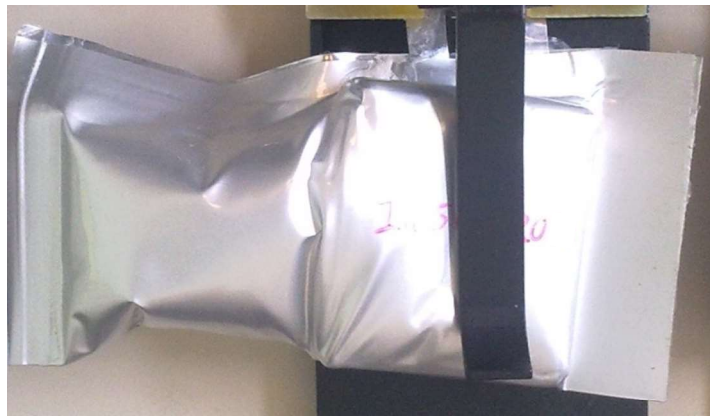
Figure 2: Photograph of a LNM/LTO pouch cell after 118 cycles between 1.5 and 3.5 V at 20°C and a C/5 rate with 2% of GA additive.
