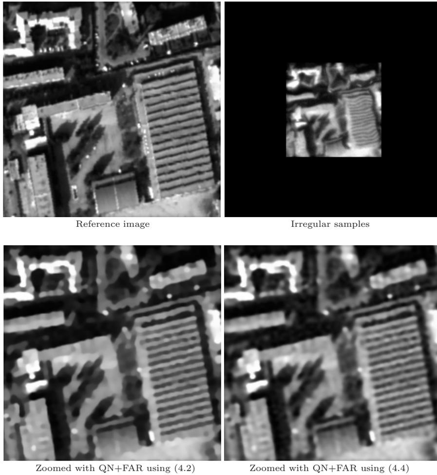
FIG. 8.9. *Deconvolution denoising and zoom. We display the QN+FAR results using a spectral decay like:  $(\frac{2\pi\omega}{N})^{1.6}$ , which coincides with the decay of the reference image. The stair-casing effect in (c) (RMSE: 6.003) is due to the poor discretization of the regularizer in (4.2). In (d) (RMSE: 5.957) we observe the result obtained with a finer discretization of the regularizer (4.4).*
