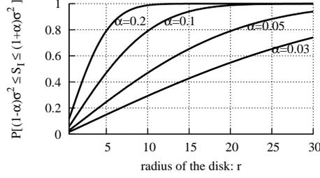
FIG. 7.2. Relation between the expected number of satisfied constraints and the radius  $r$  of the disk used for the local noise estimation. The graph shows the curves computed for different widths of the band  $\alpha$ .
