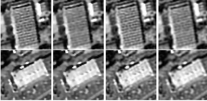
FIG. 8.6. Two details of images deconvolved using total variation and  $L^2$ -norm of the gradient as regularizers, both with local and global constraints. From left to right is shown the result of the proposed algorithm (4.4), ACT+TV [5] (global constraint), the  $L^2$ -norm with local constraints and with a global constraint. Note that the last two results are more blurred than the total variation ones, and as seen in Table 8.2 have a higher RMSE.
