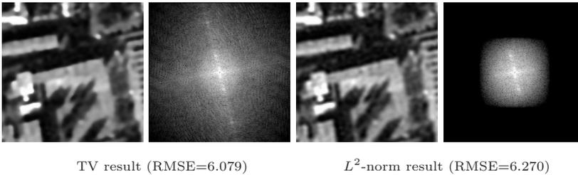
FIG. 8.8. Deconvolution and zoom using TV and the  $L^2$ -norm of the gradient as regularizers. The images show a detail of the zoomed images and its spectrum. Note that the  $L^2$  regularizer recovers the low frequencies but is unable to extrapolate to higher ones.
