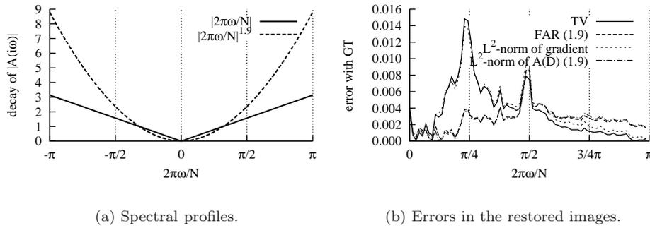
FIG. 8.3. Denoising experiments with different selections of spectral profiles  $A(i\omega)$ . Using the spectral profile that fits the model for the ground truth image, reduces the error, especially in the mid-low frequencies.
