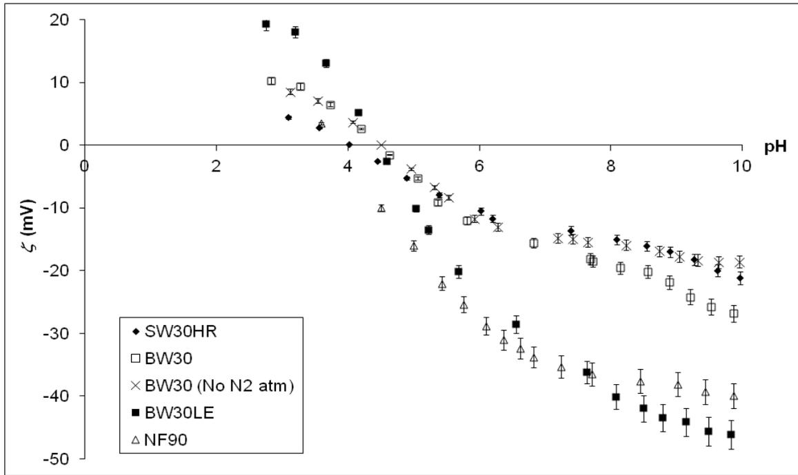
**Fig. 4:** pH dependence of zeta potential of NF90, BW30LE, BW30 and SW30HR membranes; For the BW30 membrane, measurements were also performed without controlled atmosphere (cross symbols). Error bars correspond to two successive measurements.
