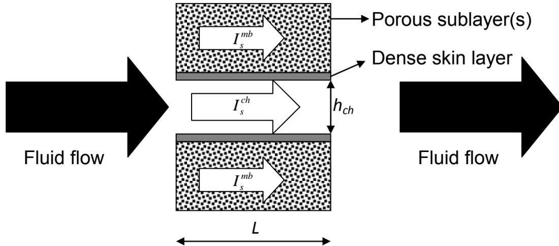
**Fig.1:** Distribution of the streaming current during tangential electrokinetic experiments with membranes whose porous structures are exposed to the hydrodynamic fluid flow.  $I_s^{ch}$  is the streaming current flowing through the channel,  $I_s^{mb}$  the streaming current flowing through the porous sublayer(s) of the membrane samples,  $L$  is the sample length, and  $h_{ch}$  is the channel height.
