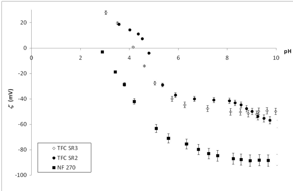
**Fig. 5:** pH dependent zeta potential curves of NF270, TFC-SR2 and TFC-SR3 membranes. Error bars correspond to two successive measurements.
