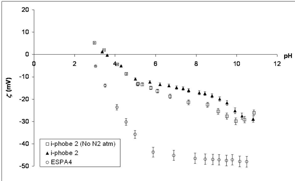
**Fig. 7:** pH dependent zeta potential curves of ESPA4 and i-phobe 2 measured under  $N_2$  atmosphere. For i-phobe 2 membrane, measurements were also performed without controlled atmosphere (square symbols). Error bars correspond to two successive measurements.
