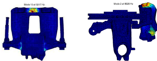
Figure 12. A free/free caliper mode and its projection on the time model. Color code: Left, strain energy. Right, displacement.
