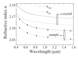
FIG. 4. Dispersion curve of the refractive index in both polarization and comparison with the single crystal values. <sup>15</sup>
