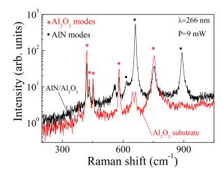
FIG. 2. MicroRaman spectra collected from w-AlN/Al $_2O_3$  film. Red line is related to Al $_2O_3$  substrate microRaman spectrum, as the black one to AlN on Al $_2O_3$ . The squares are assigned to w-AlN modes and the stars are assigned to Al $_2O_3$  substrate modes.
