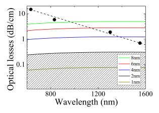
FIG. 7. Evolution of propagation losses at different wavelengths (dots) and calculated scattering optical losses as a function of the wavelength for m=0 and for different values of rms roughness (curves) for TE polarization.
