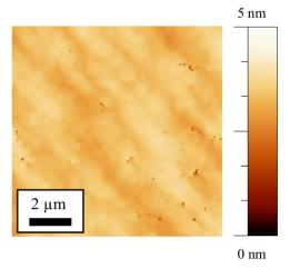
FIG. 8. AFM 2D mapping of the AlN surface sample. The average calculated rms roughness value is 2 nm.
