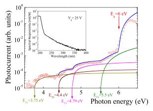
FIG. 3. Spectral photocurrent of an AlN MSM photodiode measured at  $\pm 5\,\mathrm{V}$  bias. The inset shows the spectral responsivity (mA/W) at  $+25\,\mathrm{V}$  bias between the MSM interdigitated electrodes.
