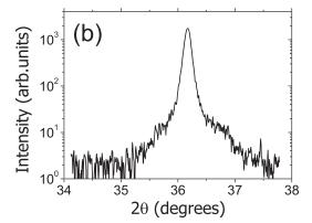
FIG. 1. XRD spectra of AlN film on Al<sub>2</sub>O<sub>3</sub> substrate (a) in the  $\theta$ - $\theta$  mode and (b) in the  $\theta$ - $2\theta$  rocking curve mode.
