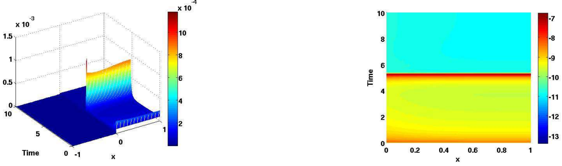
Figure 6: Evolution of the torque \|\vec{s} \times \vec{m}\|^2 during the time: 3D view (left), and with a logarithmic scale in the thin material (right).
