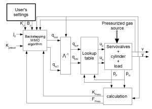
Fig. 2. Complete principle of the control strategy
