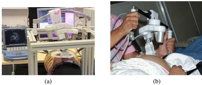
Fig. 9. Experiment setup with the PROSIT robot interacting with (a) the abdominal phantom and (b) human volunteer.
