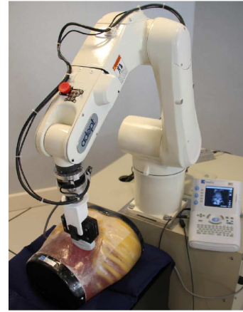
Fig. 7. The first experimental setup is composed by a 6-DOF anthropomorphic Viper (Adept) robot holding a US probe that interacts with a realistic abdominal phantom
