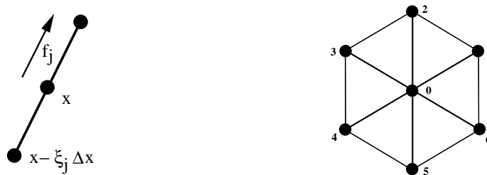
Figure 1. Typical stencil of a lattice Boltzmann scheme for a Bravais lattice (left) ; both opposite directions \xi_j and -\xi_j connect two vertices of the mesh. Local numbering of the six neighbours (right) of the D2T7 lattice Boltzmann scheme on triangles.
