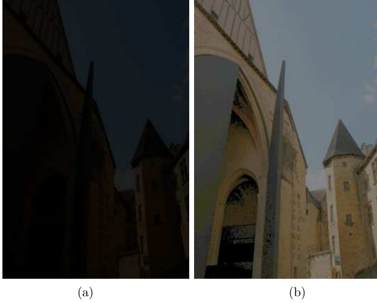
Figure 20: (a) initial image with low lighting conditions, (b) corrected image with dynamic centring by optimal \lambda_0
