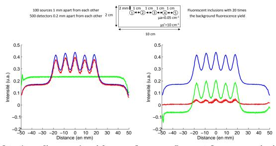
Figure 5. Intensity profiles comparison: left: — raw fluorescence F, - - - autofluorescence, — local parameters fit of the fluorescence  $M_1$ , — global parameters fit of the fluorescence  $M_2$ ; right: — F, —  $(F - M_1)$ , —  $(F - M_2)$ .
