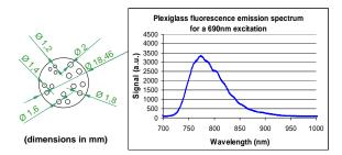
Figure 2. Spatial position and dimension of the target (left) and its fluorescence emission spectrum for a 690 nm excitation (right).
