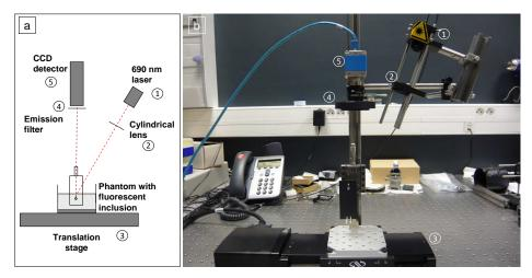
Figure 1. Optical setup used during the study (schematic (a) and platform (b)).
