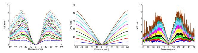
Figure 3. A/E intensity ratios obtained for increasing levels of autofluorescence with the Monte-Carlo method (left), with NIRFAST (center), experimentally (right).
