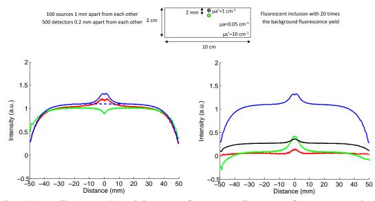
Figure 9. Intensity profiles comparison: left: — raw fluorescence F, - - - autofluorescence, — local parameters fit of the fluorescence  $M_1$ , — global parameters fit of the fluorescence  $M_2$ ; right: — F, —  $(F - M_1)$ , —  $(F - M_2)$ .
