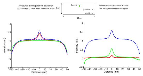
Figure 4. Intensity profiles comparison: left: — raw fluorescence F, - - - autofluorescence, — local parameters fit of the fluorescence  $M_1$ , — global parameters fit of the fluorescence  $M_2$ ; right: — F, —  $(F - M_1)$ , —  $(F - M_2)$ .
