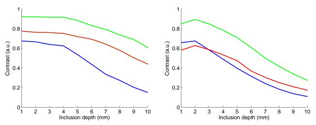
Figure 7. Comparison between the contrasts obtained with WF-FRI (-), the local parameters fitting method (-) and the global parameters fitting method (-) for a realistic background fluorescence level (left) and a stronger background fluorescence level (right) used to test the limits of the method.
