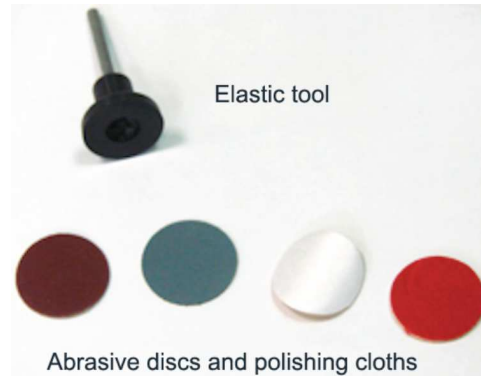
Figure 10 Description of the polishing tool (see online version for colours)
