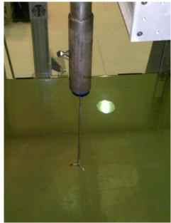
Fig. 5. Acoustic Doppler probe.
