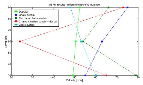
Fig. 11. ASFM velocity profiles for different types of turbulence compared to Doppler results.
