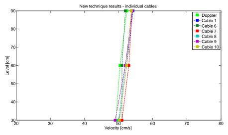
Fig. 10. Velocity profiles calculated using the new technique compared to the Doppler probe results.
