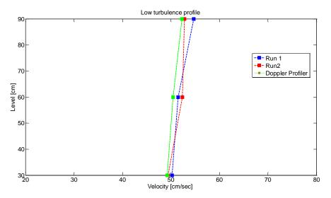
Fig. 8. Flow velocity profiles (blue and red traces) calculated using the new algorithm compared with the Doppler reference (green trace). (natural turbulence)
