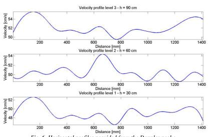
Fig. 6. Horizontal profiles provided from the Doppler probe.
