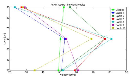
Fig. 9. Velocity profiles calculated by the ASFM compared to the Doppler probe results.
