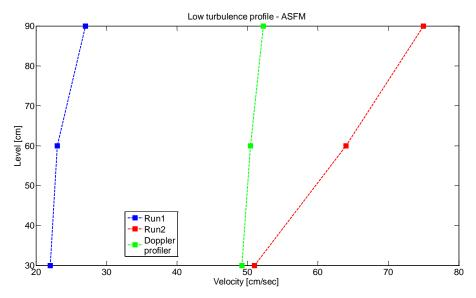
Fig. 7. Flow velocity profiles (blue and red traces) compared with the Doppler reference (green trace).(natural turbulence)
