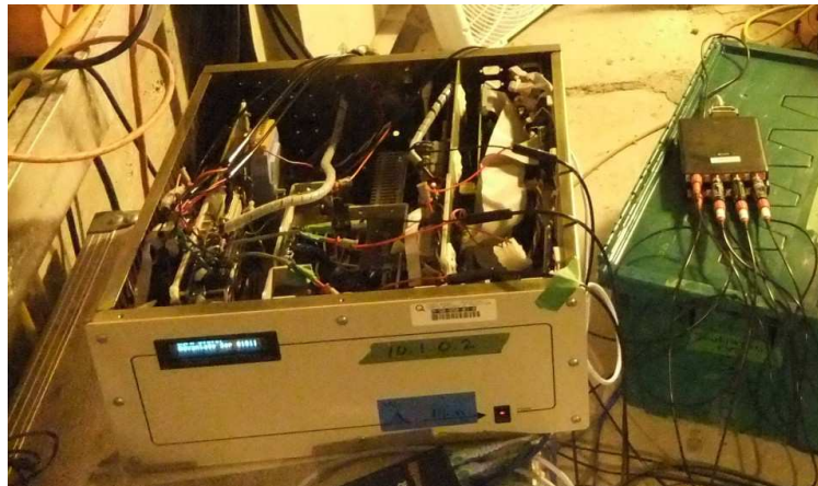
Figure 4. Data is being recorded from the ASFM using two HS4DIFF units (on the right).
