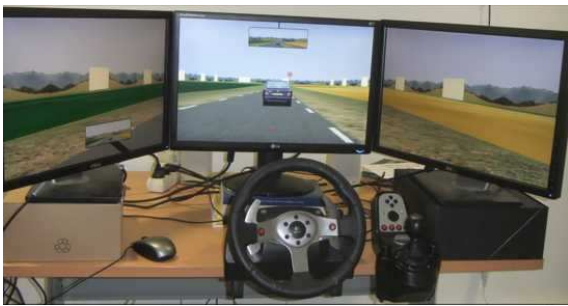
Figure 2: Driving simulator device with 3 screens, steering wheel, gearbox and a set of pedals.
